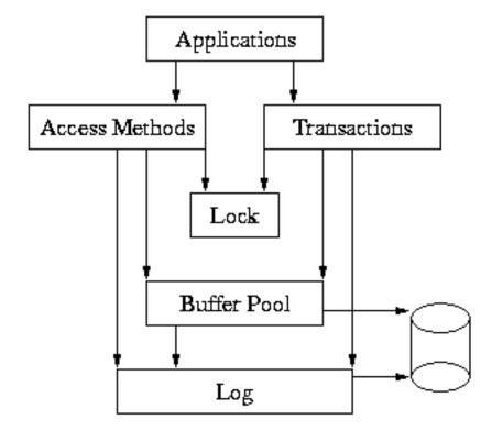
In this model, the application makes calls to the access methods and to the Transaction subsystem. The access methods and Transaction subsystems in turn make calls into the Memory Pool, Locking and Logging subsystems on behalf of the application.
